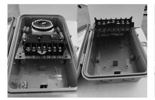
The ICM550 correctly placed in channels (A) with screw holes secured using the four plastic standoffs (B) of the enclosure. Firmly press the board down with thumbs on both sides "\*\*\*" of "C".
