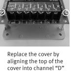
then press the bottom of the cover down firmly until it snaps into place.
